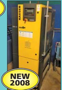
15 HP Kaeser Model Aircenter SM15 Rotary Screw Air Compressor
