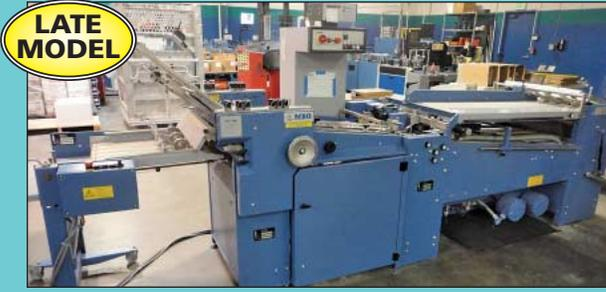
MBO Type B21-1-21/4 Continuous Feed Folding Line
