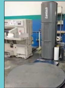
Lantech Model Q Series Semi-Automatic Pallet Stretch Wrap Machine
