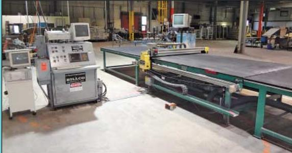
78" X 120" Billco Two-Axis Bridge Type CNC Glass Cutting Table
