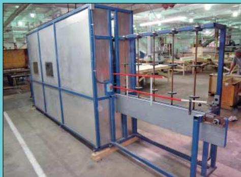
30" High Custom Built Vertical Continuous Feed Glass Panel Air Dryer
