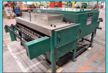
60" Wide Billco Swiggle Type Insulated Glass Electric Heated Roller Press
