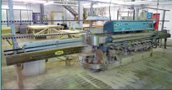
Bovone Electromeccanica Model Mini-Max 371 Pass-Thru Vertical Edge Class Beveler
