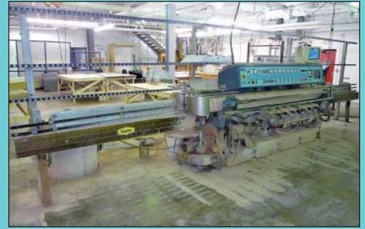
Bovone Electromeccanica Model Mini-Max 371 Pass-Thru Vertical Edge Glass Beveler
