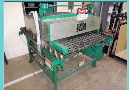
36" Wide Billco Model 3-266-074 Swiggle Type Insulated Glass Electric Heater Roller Press
