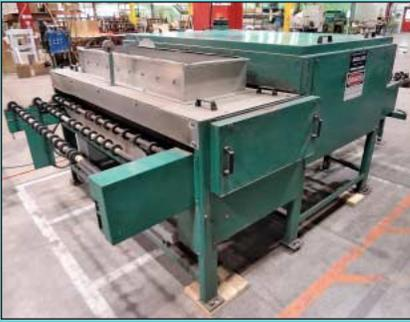
60" Wide Billco Swiggle Type Insulated Glass Electric Heated Roller Press
