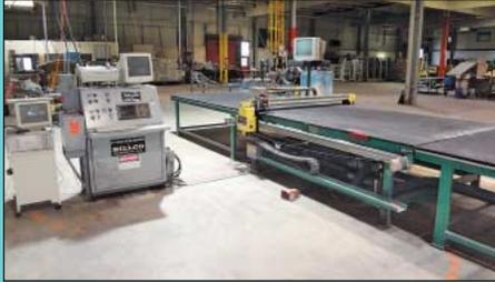
78" X 120" Billco Two-Axis Bridge Type CNC Glass Cutting Table
