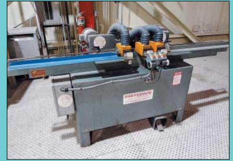
Pistorius Model S-Drill Three-Spindle Stile Drill
