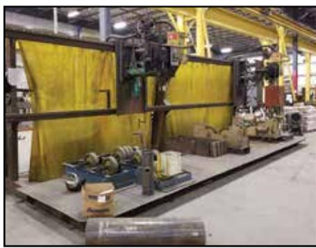
30' 2-Head Beam Sub-Arc Welder
