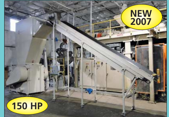
(2) 36" X 36" Rotogran Model WO-3636-HD-TB Plastic Granulators
