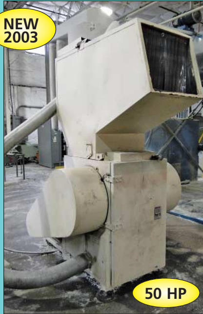
22" X 24" Rotogran Model WO-2224 Plastic Granulator
