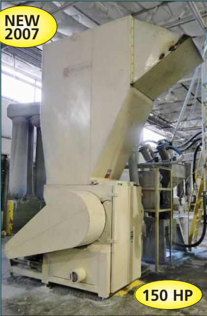
(2) 36" X 36" Rotogran Model WO-3636-HD-TB Plastic Granulators
