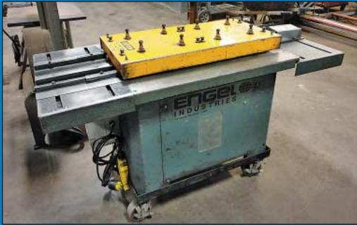
20 Ga. Engel Model M-800-S S-Drive & Snap Lock Rollformer
