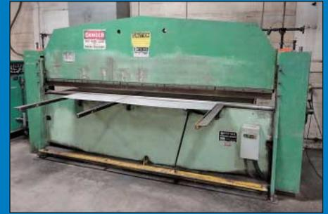
10 Ga. X 10' Roto-Die Model 15 Hydraulic Press Brake
