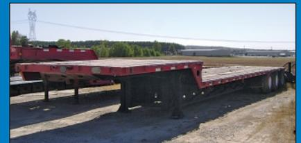
40 Ton Transcraft Model DTL-3-19-44 Tri-Axle Step Deck Trailer
