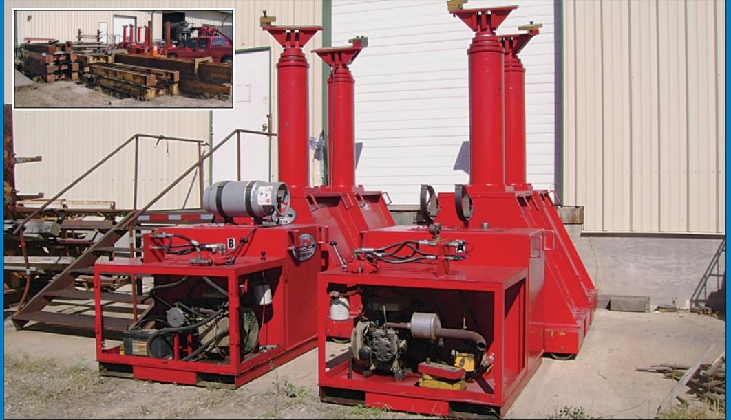
400 Ton Lift Systems Model 44A Four-Point LP Gas Hydraulic Gantry System
