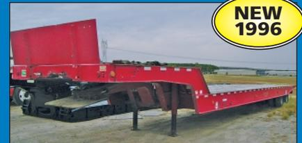
25 Ton Max Landoll Hauloff Tandem Axle Tilt Bed Trailer w/ Winch
