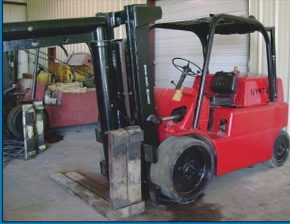
15,000 LB Hyster Model S-150 Diesel Power Solid Tire Lift Truck
