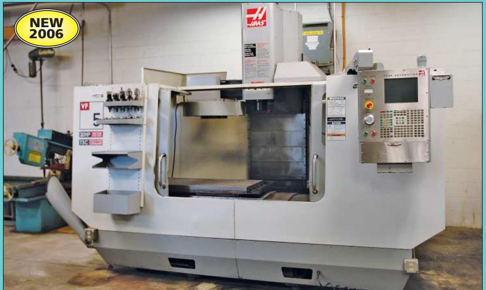
Haas Model VF-5D/40 CNC Vertical Machining Center
