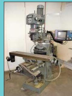
3 HP Lagun Model FTV-2 Variable Speed Vertical Milling Machine
