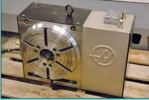
12" Haas Model HRT310 Version P3 CNC Rotary 4th Axis
