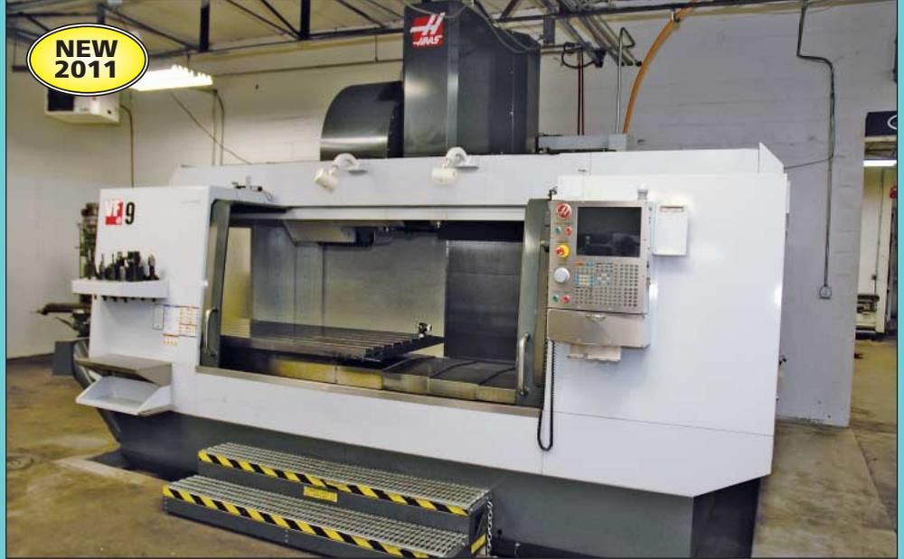
Haas Model VF-9/50 CNC Vertical Machining Center
