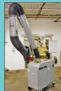
Smog-Hog Model Porta Clean Portable Fume Collector
