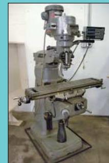
2 HP Bridgeport Variable Speed Vertical Milling Machine
