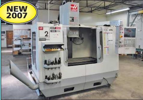
Haas Model VF-2D/YT CNC Vertical Machining Center
