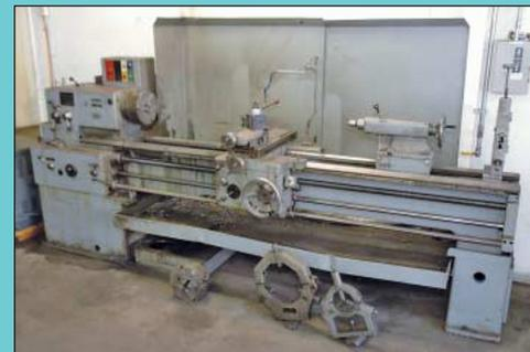
22" X 80" TOS Type SN50B Gap Bed Geared Head Engine Lathe
