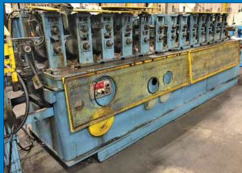
(5) Dahlstrom Thirteen and Twelve Stand Rollformers
