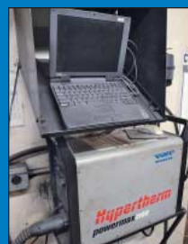
Close Up View of Control and Power Supply For Plasma Table
