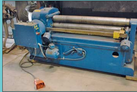
8 Ga. X 5' Webb Three-Roll Power Rolls
