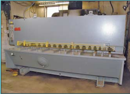
1/2" X 10' Atlantic Model HD50-10 Hydraulic Power Squaring Shear
