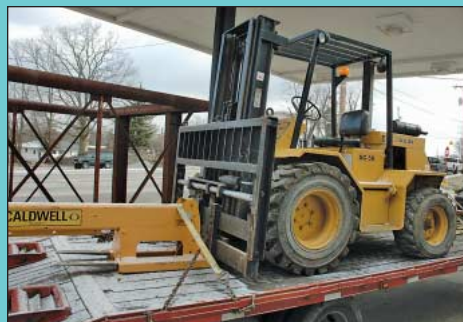
5,000 LB Sellick Model SC-50 Rough Terrain LP Gas Lift Truck
