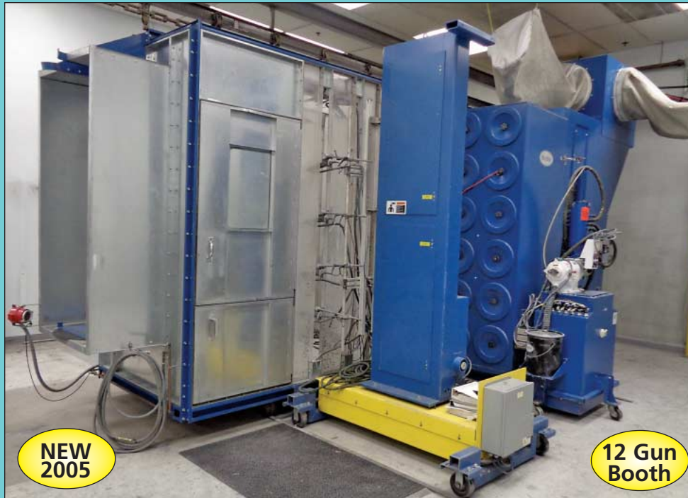
(3) Nordson Model XL-2001 Eight-Gun Automatic Poly Upper Pass-Thru Powder Coat Booths
