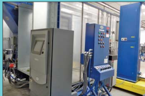
Nordson Model XL-2001 Twelve-Gun Automatic Pass-Thru Powder Coat Booth
