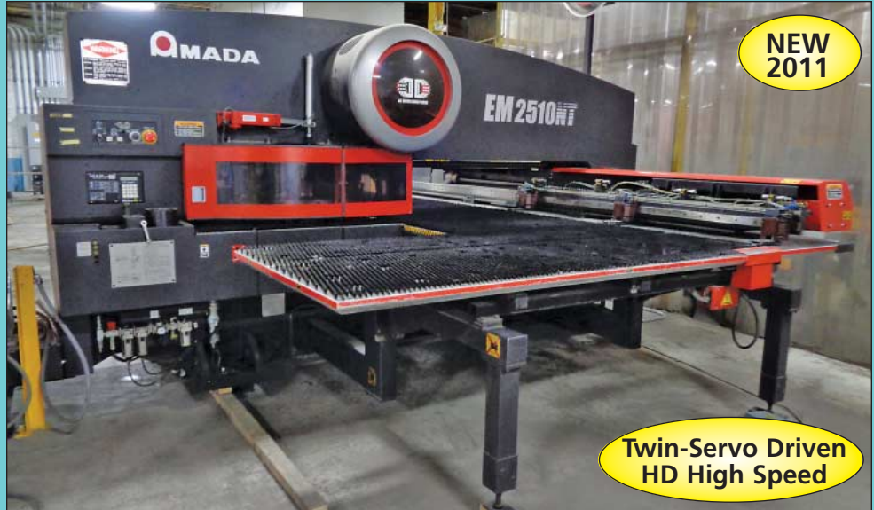
22 Ton Amada Model EM-2510NT Electric Power Twin Servo Driven Heavy Duty High Speed CNC Turret Punch
