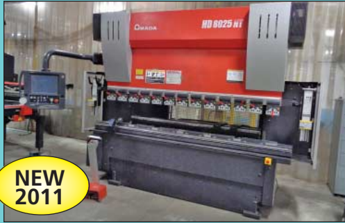
88 Ton x 101" Amada Model HD8025NT CNC Press Brake
