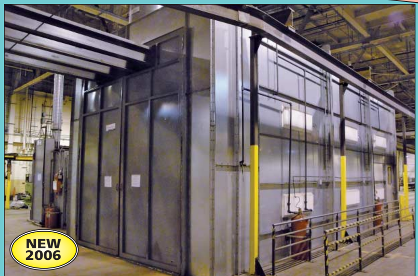
16' Wide X 34' Long X 14' High Global Finishing Solutions Model CDG-1616-NDT Crossdraft Drive Type Paint Booth
