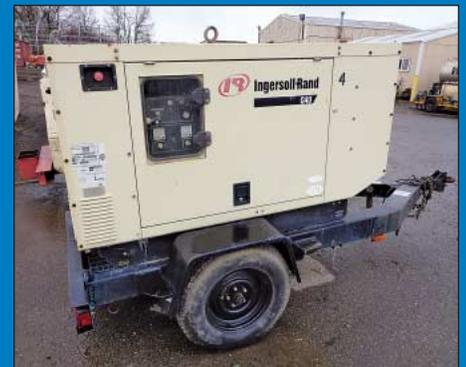
33 KW Ingersoll Rand Model G40 Diesel Power Portable Gen Set
