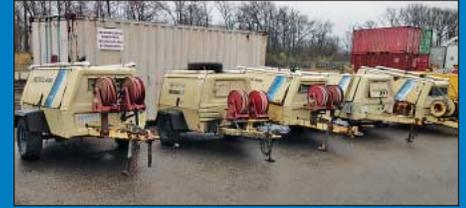
(5) Ingersoll Rand Model P175 & P185 Portable Air Compressors
