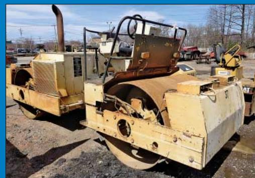
Ingersoll Rand Model DD90 Sit Down Type Smooth Drum Vibratory Roller
