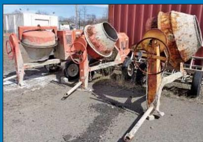
(4) Stone Model 95CM Portable Gas Powered Cement Mixers
