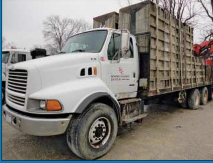
2000 Sterling Model LT9513 Tandem Axle Concrete Form Delivery Truck w/ Fassi Hydraulic Crane
