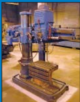
3' Arm X 9" Column Cincinnati Bickford Radial Arm Drill
