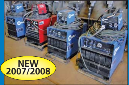
(18) 450 Amp Miller Dimension 452 Mig Welders with Miller 22A and 24A Wire Feeders
