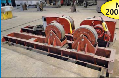
(5) 45 Ton / 30 Metric Ton Romar Model PR30/45DM Motorized Tank Turning Roll Sets w/ Idlers
