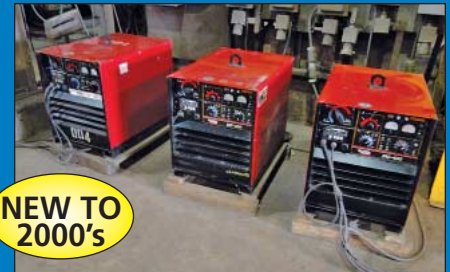
(32) 400 Amp Lincoln Idealarc DC-400 Mig Welders with Lincoln LF72 and LN7 Wire Feeders
