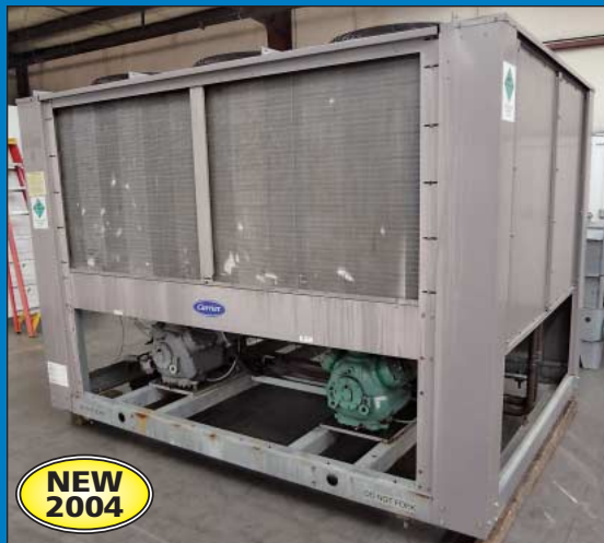
70 Ton Carrier Model 306TN070-631KA Air Cooled Chiller
