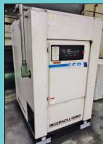
50 HP Ingersoll Rand Model SSR-EP50 SE Rotary Screw Cabinet Type Air Compressor
