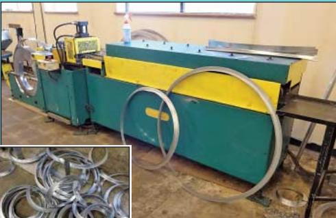
6" Ovalformer 12-stand Rollformer w/ Shear & Uncoiler
