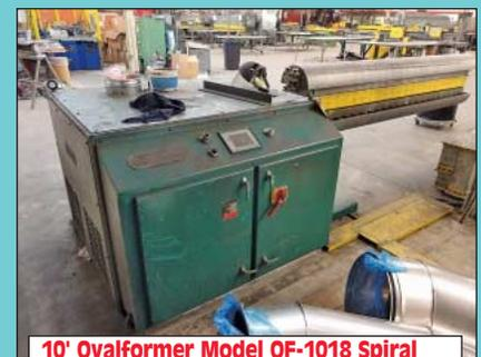
10" Ovalformer Model OF-1018 Spiral Duct Tube Ovalizer
