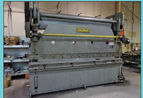
12' Cincinnati Series 90-10 Mechanical Power Press Brake
