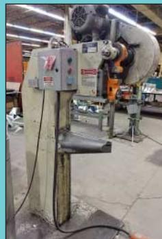
6 Ton Azimuth and Taloc Model H412 Clinching Machines
