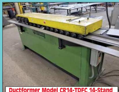
Ductformer Model CR14-TDFC 14-Stand TDF Rollformer
