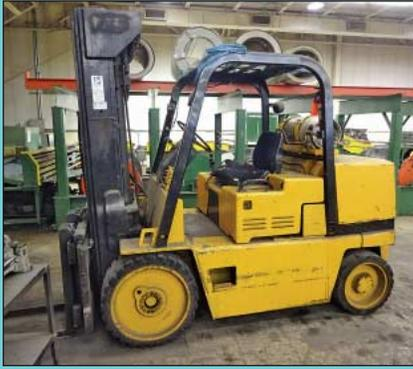
12,500 Lb. Caterpillar Model T125D Solid Tire LP Gas Lift Truck
