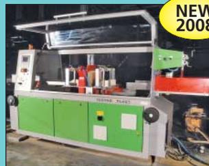
Techno-Plast Model Profitec-SA-1 Automatic Up-Acting Saw
