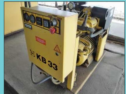
30 HP Ingersoll Rand Model KB33 Rotary Screw Skid Mounted Air Compressor
