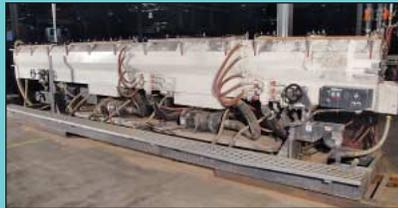
(2) Conair Model MSB20S Spray Vacuum Calibration Tanks
