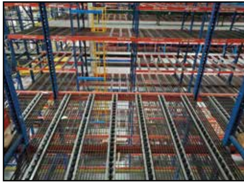
(2) Tear-Drop Style Pick Modules w/1,467 Half-Pallet & 844 Full-Pallet Locations, Power Belt Conveyors & Gravity Feed Rack
