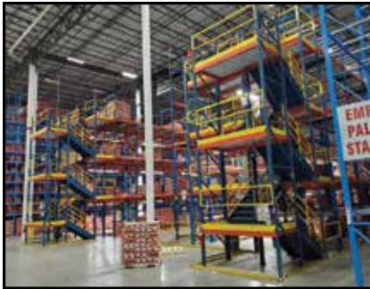
(2) Tear-Drop Style Pick Modules w/1,467 Half-Pallet & 844 Full-Pallet Locations
