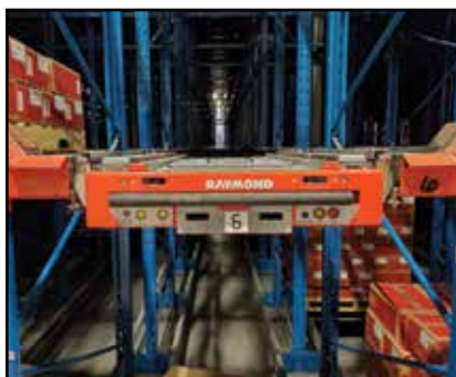
RAYMOND Push-Back Rack Shuttle Systems w/(6,000) Pallet Spaces, Shuttles & Rechargeable Battery Systems
