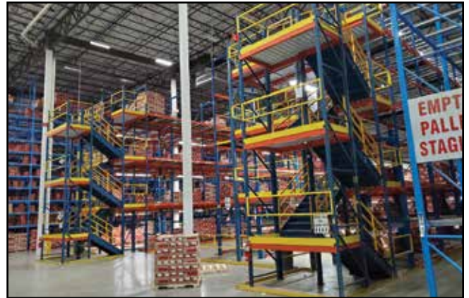
(2) Tear-Drop Style Pick Modules w/1,467 Half-Pallet & 844 Full-Pallet Locations
