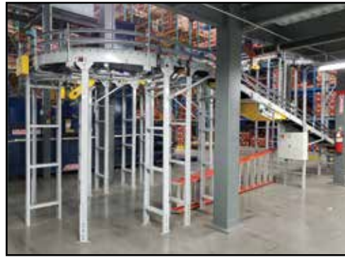
(2) Tear-Drop Style Pick Modules w/1,467 Half-Pallet & 844 Full-Pallet Locations, Power Belt Conveyors & Gravity Feed Rack
