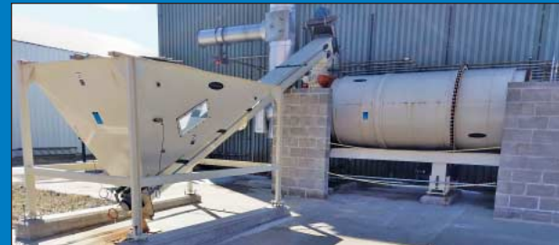
4' Dia. x 12' Long EcoTherm E-450x22 Three-Pass Rotary Drum Dryer w/ Metering Feed Hopper, Auger Conveyor
