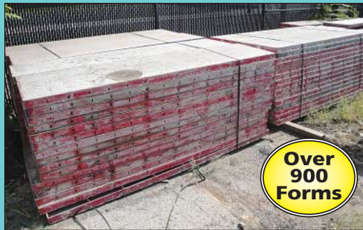
Partial View of (140) 24" X 96" Symon Steel Frame/Smooth Plywood Concrete Forms
