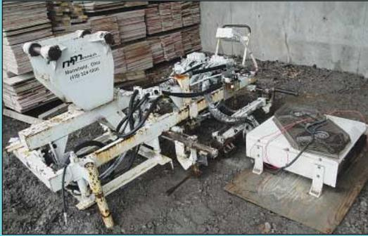
Minnich Model H-3 Three-Spindle Gang Drill Attachment
