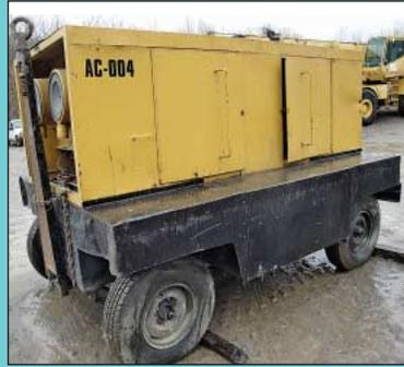
Sullair Model 750-DP Trailer Mount Diesel Power Portable Air Compressor
