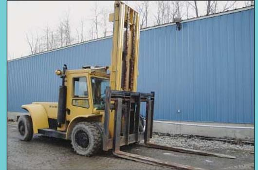
30,000 Lb Hyster H300B Dual Pneumatic Tire Diesel Power Lift Truck
