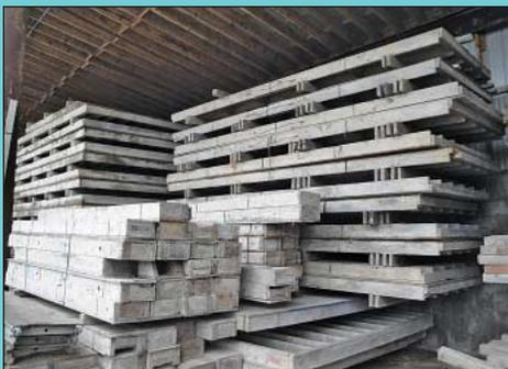
Large Quantity Ohio & Pennsylvania Spec Wall & Barrier Forms Up to 16' X 10' Wall Forms
