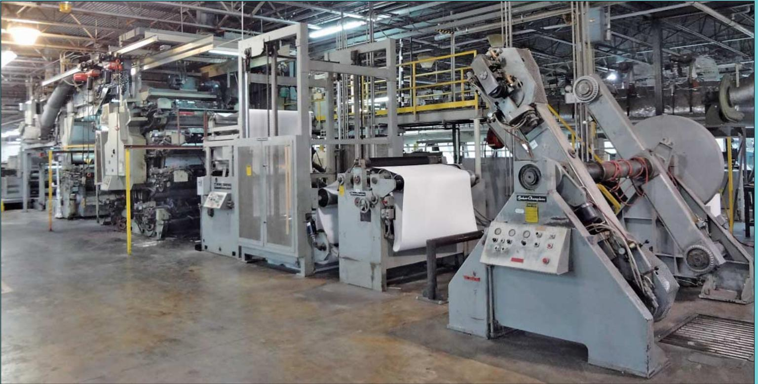
55" Wide Kidder-Stacey Model 660Z Centraflex / Bobst Champlain Lemanic S1425 8-Color Roll to Sheet Central Impression Flexographic Printing Press Line
