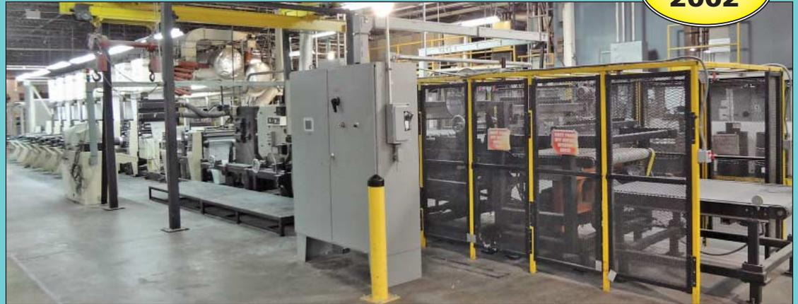
28" X 36" Comco Model Mark IV 8-Color Roll to Sheet Inline Narrow Web Flexographic Printing Press Line
