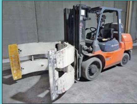
12,000 LB Toyota LP Gas Lift Truck w/ 7,700 LB Cascade Roll Clamp Attachment
