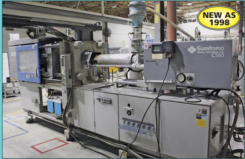
(2) 180 Ton X 9 Oz. Sumitomo Model SG180M-H Toggle Clamp Plastic Injection Molding Machines
