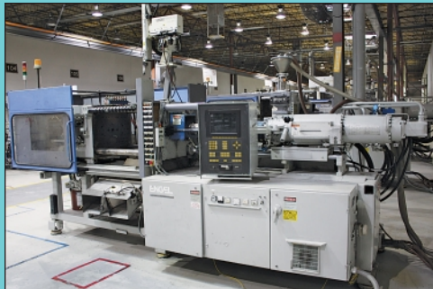
200 Ton X 13.2 Oz. Engel Model ES700/200 Toggle Clamp Plastic Injection Molding Machine
