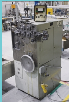
(2) Torrington Model W11A Spring Winders
