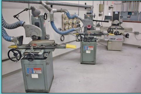
(2) 6" X 18" Boyar Schultz Model HR618 Hand Feed Surface Grinders
