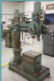
3' Arm X 9" Column Arborga Radial Arm Drill
