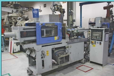
55 Ton X 3.1 Oz. Arburg Model 270-210-500 Toggle Clamp Plastic Injection Molding Machine
