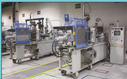
(2) 85 Ton X 3.5 Oz. Demag Model D85NCII Toggle Clamp Plastic Injection Molding Machines
