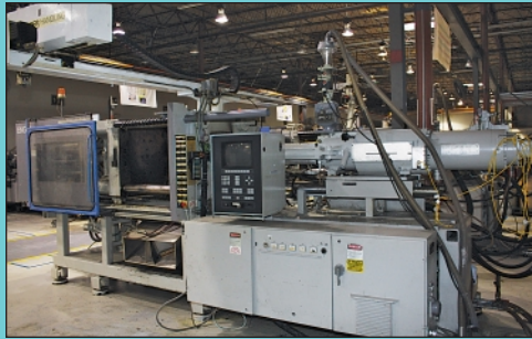
(3) 300 Ton X 23.34 Oz. Engel Model ES1300/300 Toggle Clamp Plastic Injection Molding Machines
