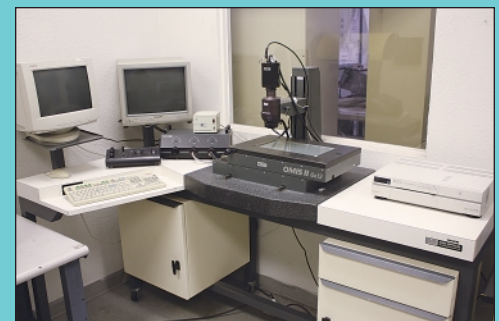
6" X 12" Ram Optical Model OMIS II CNC Optical Video Probe Inspection Machine
