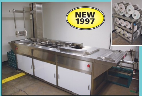
Crest Model OC5-1218-HC Five-Station Automatic Dip Ultrasonic Parts Washing Line
