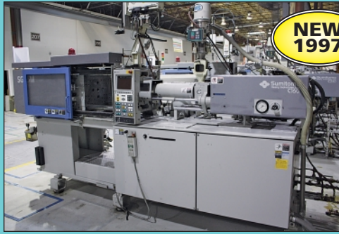
75 Ton X 4 Oz. Sumitomo Model SG75M-H Toggle Clamp Plastic Injection Molding Machine
