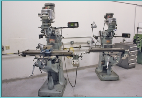
(3) 2 HP Bridgeport Vertical Milling Machines
