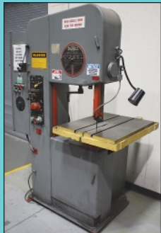
20" DoAll Model 2012-2H Metal Cutting Vertical Band Saw
