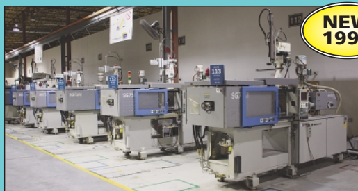
Bank View (5) 75 Ton Sumitomo Model SG75M-H Plastic Injection Molding Machines
