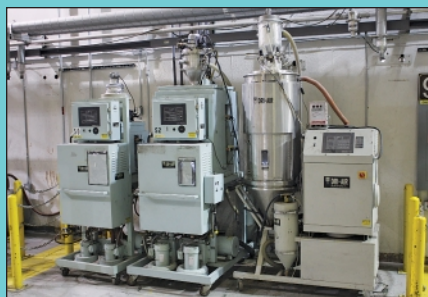
(4) Dri-Air Model Arid-X 50PD Dehumidifying Dryer And Hopper Systems
