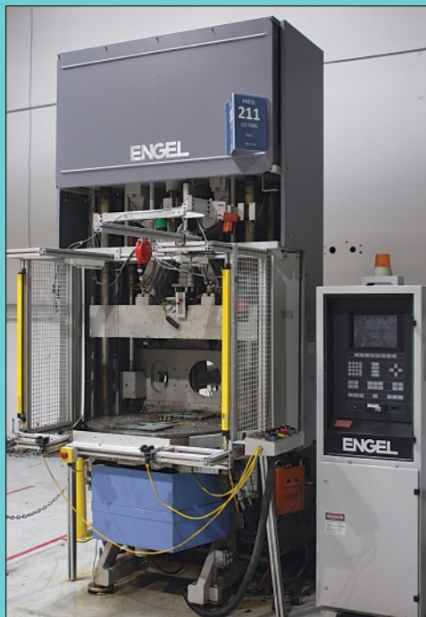
125 Ton X 8 Oz. Engel Model ES330/150VHRT Vertical Rotary Table Type Plastic Injection Molding Machine
