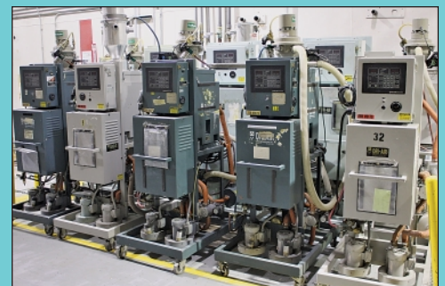
(10) Dri-Air Model Arid-X 35PD Dehumidifying Dryer And Hopper Systems
