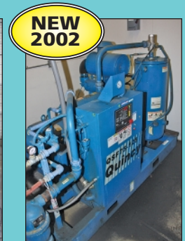
75 HP Quincy Model OSF75WNW32C Skid Mounted Rotary Screw Air Compressor
