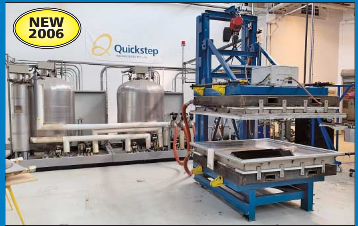
NEW 2006 Quickstep **Quickstep Out-of-Autoclave Bladder Bed Forming Composite Curing RTM & Pre-Preg 1/3 Cure Time
