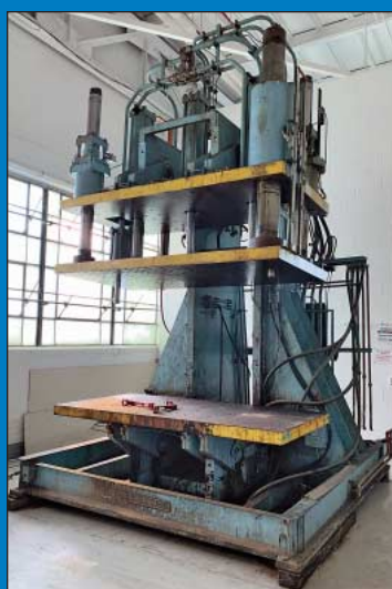
200 Ton Admiral Equipment Co. Hydraulic Booking Press for Composite Molding, RTM, Pre-Preg
