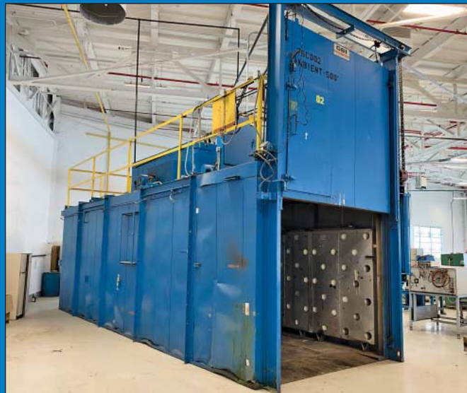
8' x 8' x 20' Deep OSI Drive-In Natural Gas Oven w/ Large Process Truck
