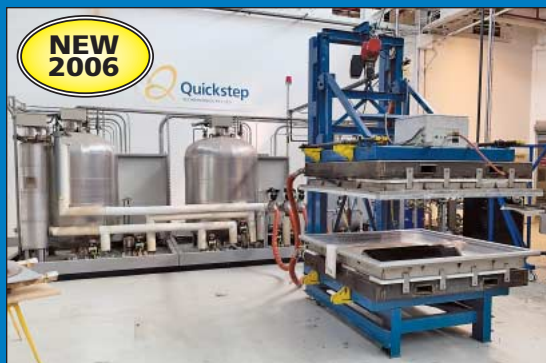
**Quickstep Out-of-Autoclave Bladder Bed Forming Composite Curing RTM & Pre-Preg 1/3 Cure Time
