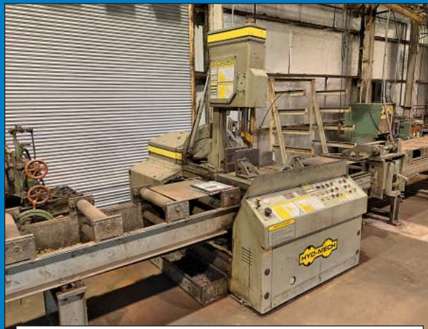
28" x 18" Hydmech Model V18 Tilt Frame Vertical Band Saw
