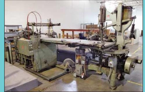
25" FMC Stokes and Smith B-Box Line Consisting of Model 405 Coater, Model RB2 Box Spotter & BP Stroke Feed
