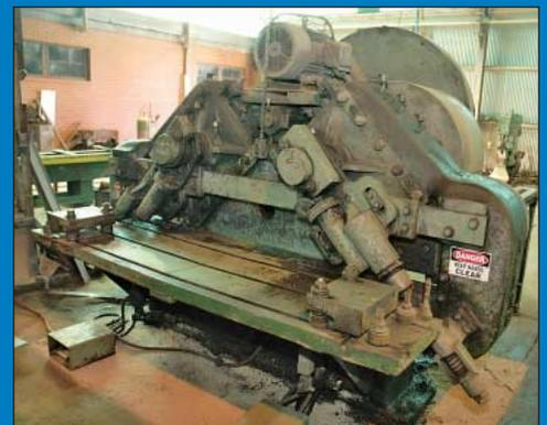
King Mechanical Bar and Angle Shear
