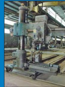
5' Arm X 11" Column American Hole Wizard Radial Arm Drill Mounted on 60" Wide X 60" Rail Track System
