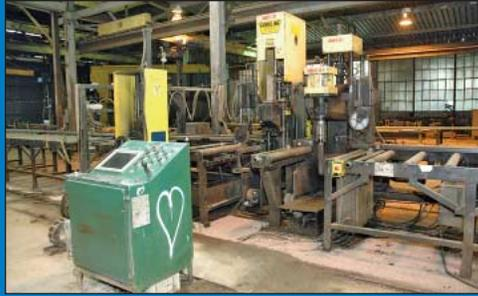
Controlled Automation Fabriline Model 3456-179 Automatic I-Beam Punch Line
