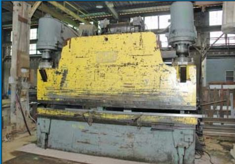
300 Ton X 12' Chicago Dries & Krump Model 300-VC10 Hydraulic Power Press Brake
