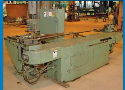
3/4" Pines Model M-725559 Horizontal Hydraulic Tube Bender
