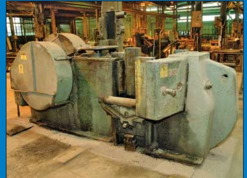
Cleveland Horizontal Bull-Dozer Forming and Straightening Press
