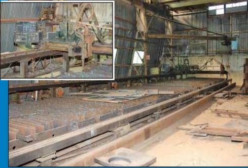
ESAB Model 200D Oxy Acetylene Three-Torch Plate Burning Table
