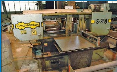
Hyd-Mech Model S-25A Mitre Base Automatic Horizontal Band Saw
