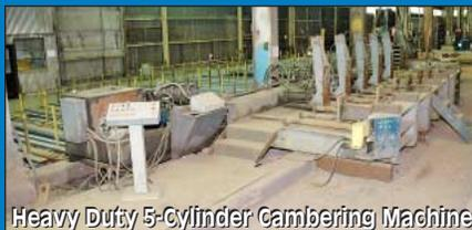
Heavy Duty 5-Cylinder Cambering Machine
