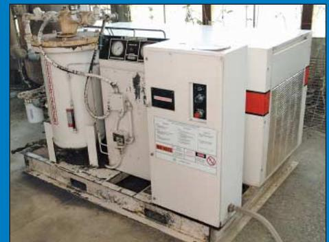
(2) 50 HP Gardner Denver Electra-Saver II Intensive Injection Rotary Screw Skid Mounted Air Compressors
