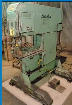
(2) 120 Ton Piranha Model SEP120 Single End Hydraulic Plate Punches
