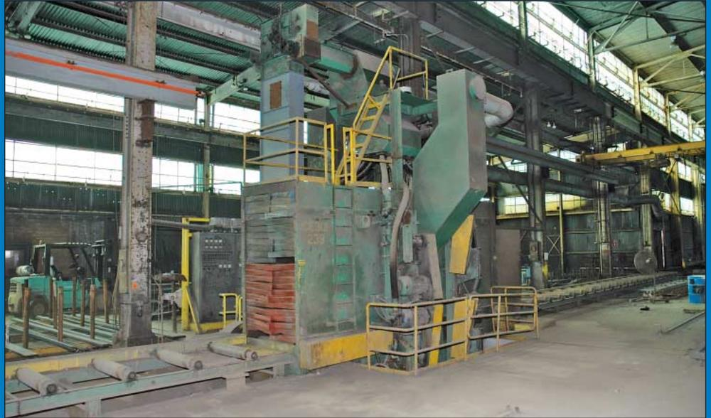
Wheelabrator Eight-Wheel Roller Conveyor Pass-Thru Shot Blast Machine
