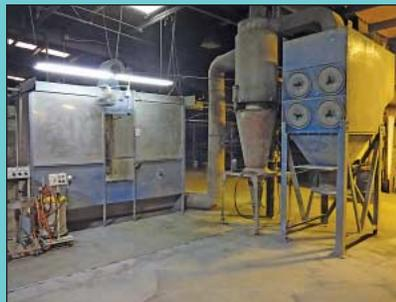
36" Wide X 10' Long X 9' High Manual Steel Pass Thru Single Station Powder Coat Spray Booth
