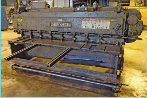
10 Ga. X 8' Cincinnati Model 1008 Mechanical Shear
