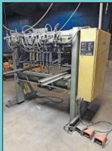
60 KVA Standard Model Special Ten-Head Ram Type Spot Welder
