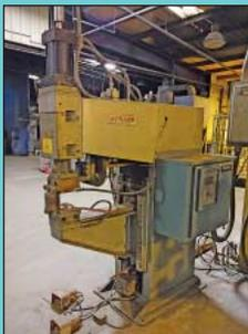
100 KVA Standard Model PP1-24-100 Ram Type Spot Welder
