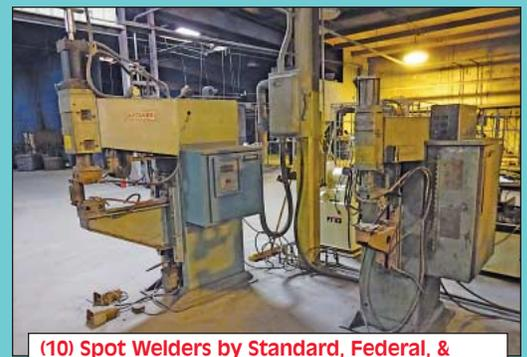
(10) Spot Welders by Standard, Federal, & Lora Up to 100 KVA
