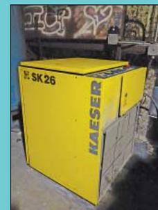
20 HP Kaeser Model SK26 Cabinet Enclosed Rotary Screw Air Compressor
