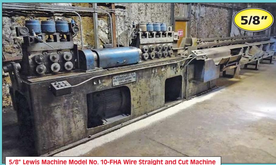
5/8" Lewis Machine Model No. 10-FHA Wire Straight and Cut Machine
